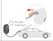
2- Place the charging cable on the socket holder of the station.
