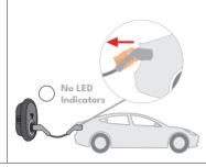
2 - Remove the charging cable from the station.
